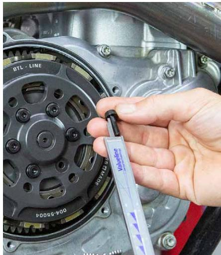
**The effective Gap is calculated as follows and corrected if necessary:**
